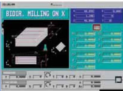
Unidirectional and bidirectional surface milling
