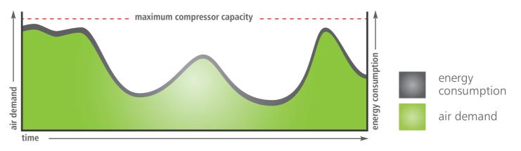
The Avelair variable speed compressors mirror the demand for air by altering the motor speed ensuring you only pay for the air you use.
