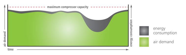
The Avelair fixed speed compressors are efficient for constant air demand users. When air demand reduces, the compressor will run offload making it less efficient to run than a variable speed compressor.
