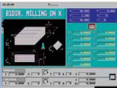
Unidirectional and bidirectional surface milling
