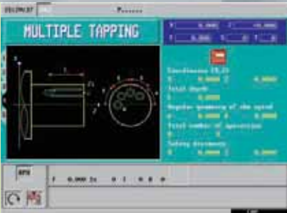
Multiple drilling and tapping
