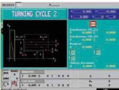
Turning, facing, taper, rounding
