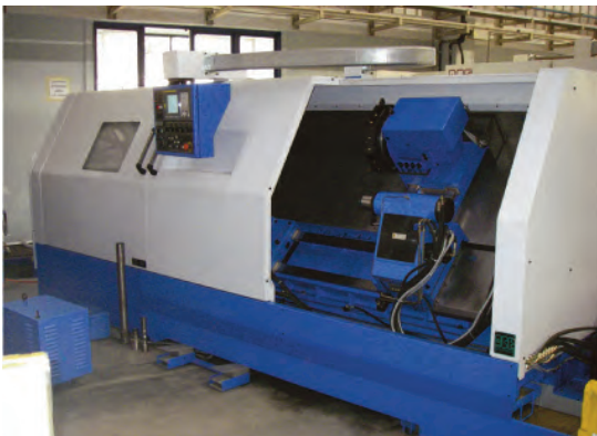
AJSBHD 300-1500 showing powered tailstock
